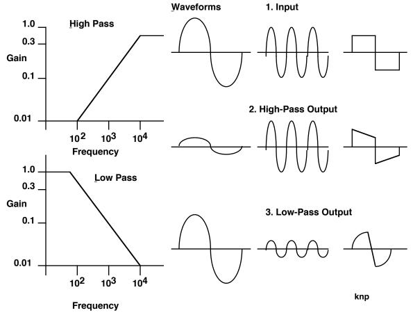
The effects of low and high pass filtering on sine waves of different frequencies and on a square wave. You should realize that a square wave is actually a complex waveform (review the information on Fourier transformations). See if the alteration of the square wave is what you would expect by each filter.
