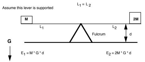
Now, suppose that both of the arms of this lever are of equal length. If we stop supporting the arms, movement will occur and useful work will be done on Mass M (#1). The energy for this work comes from gravitational pull on Mass 2 M (#2). Notice, that without the lever, this transfer of energy from a spontaneous process (the movement of mass #2 towards the earth) to a non-spontaneous process (the movement of mass#2 away from the earth) would not be possible.
